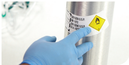
Figure 4–2: An oxygen cylinder usually has a green or white top with a yellow diamond indicating oxygen.
